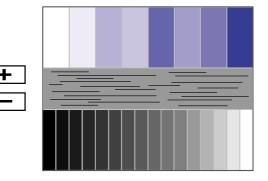
F Adjust the Phase to correct horizontal wavy noise, flicker or blur in the zebra pattern.
